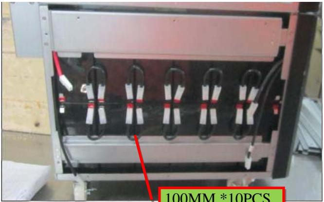
4. Connect the Batteries by 10 black wires;
